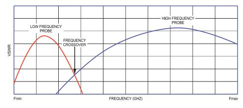
VSWR versus Frequency of a two-probe slide-screw tuner.
