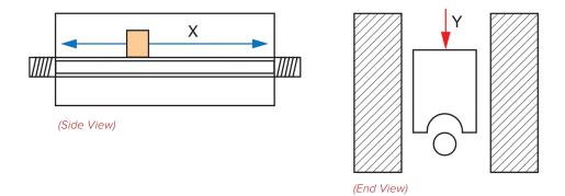
The probes used in slide-screw tuners are wideband in nature, and have similar reflective properties over a wide range of frequencies. In order to increase the overall useful bandwidth of the tuner, two probes of varying dimensions are independently used within a tuner; one for low frequencies and one for high frequencies. In this manner, it is common for slide-screw tuners to achieve an overall frequency range of several octaves to over a decade.
